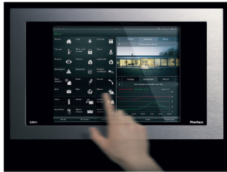
ill. Information.15.1 Touchscreen interface for controlling the building functions of a Smart Home.
